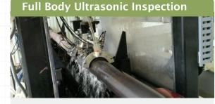
Tejas Tubular has a custom & automated Full Body Ultrasonic Inspection system to inspect its tubing pup joints.
